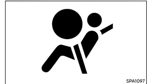
The SRS air bag warning light, displaying
